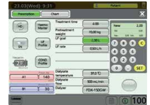
Prescription screen to reduce the touches for data entry Operators can prescribe dialysis fluid concentration with Na + and HCO 3 - in mmol.
